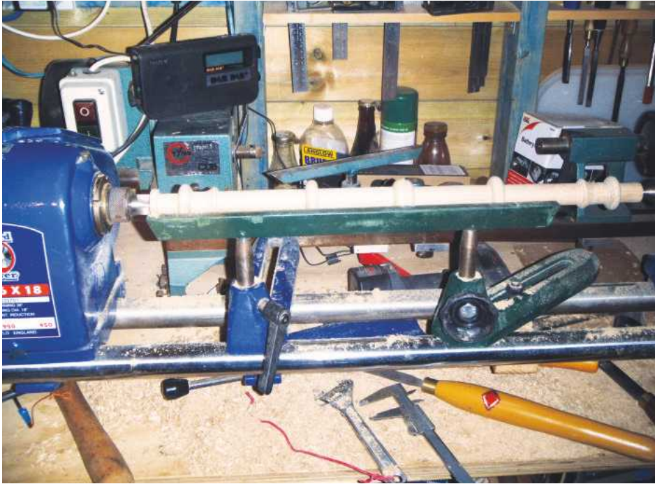
▲ Pic.5 Connecting rail being turned on the lathe
